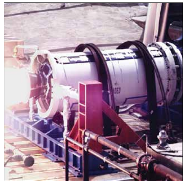
Aerojet Rocketdyne's Design Verification Test of the eSR-19. Photo courtesy of Aerojet Rocketdyne
