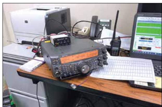
Image of a Kenwood TS-2000 Ham Radio used by those who seek a more self-sufficient mode of communication.
