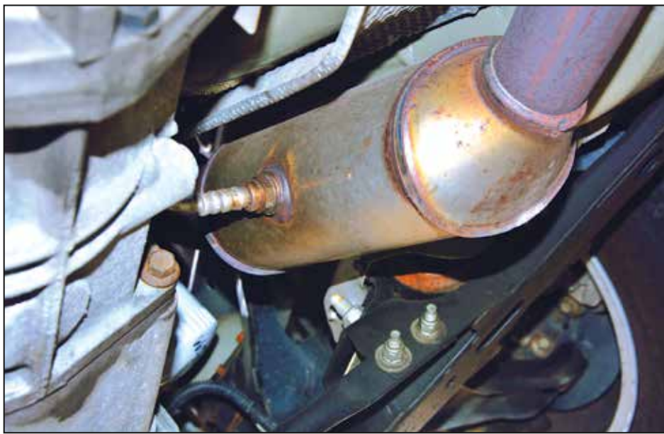
A catalytic converter is part of a vehicle's exhaust system. They often contain precious metals such as platinum, gold, rhodium, and palladium that have high value in the metal recycling market. Photo courtesy Tony Savino | Dreamstime
