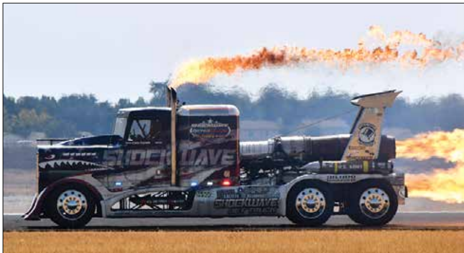
Chris Darnell's Shockwave Jet Truck, featuring three J34-48 Pratt and Whitney jet engines, is capable of over 300 mph. Photo by Rick Sloan
