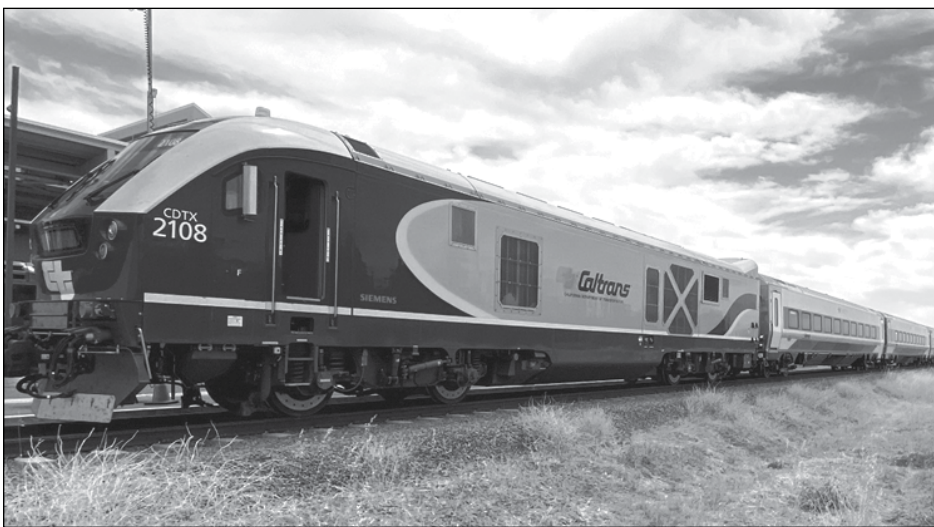
Charger locomotive leading a Siemens Mobility Venture trainset. Photo courtesy of Caltrans
