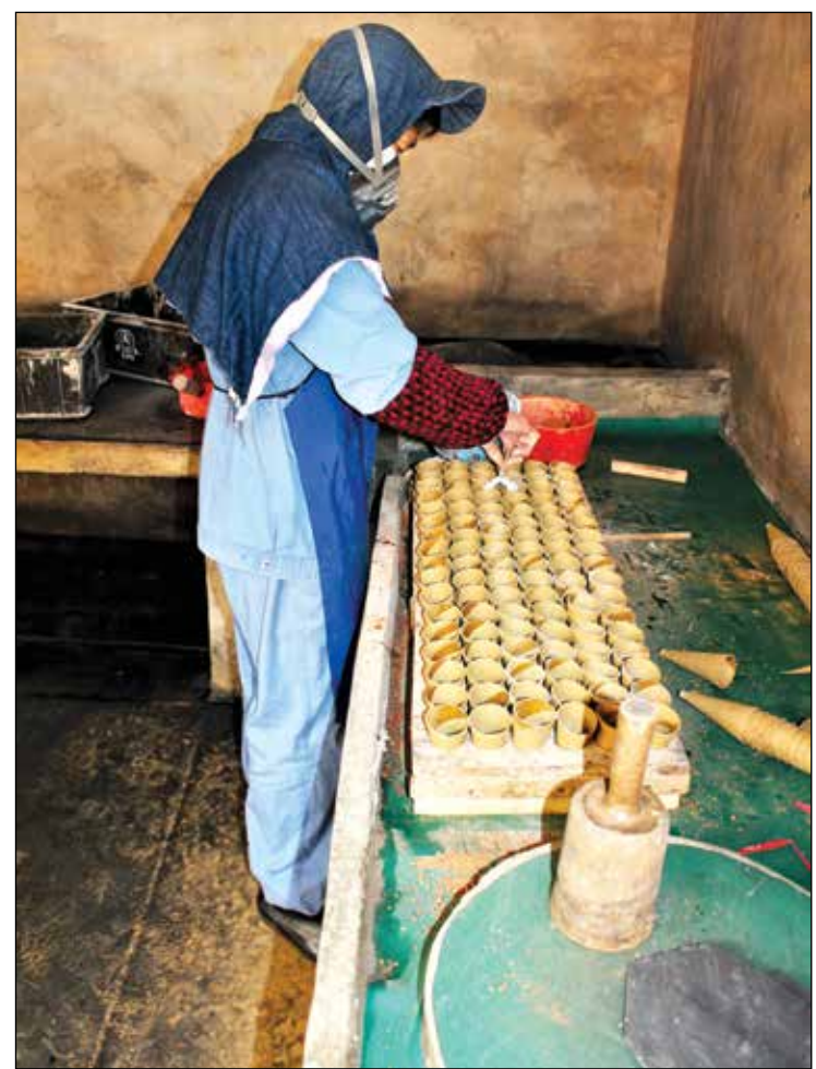
Explosive black powder is carefully handled in bunker-like buildings inside China's fireworks factories.
