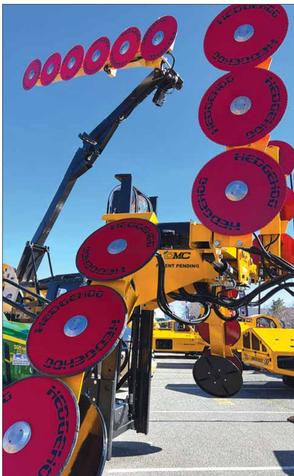
It may look like a carnival ride, but this is a hedger which takes off the tops of trees as simply as a front yard bush gets trimmed.
