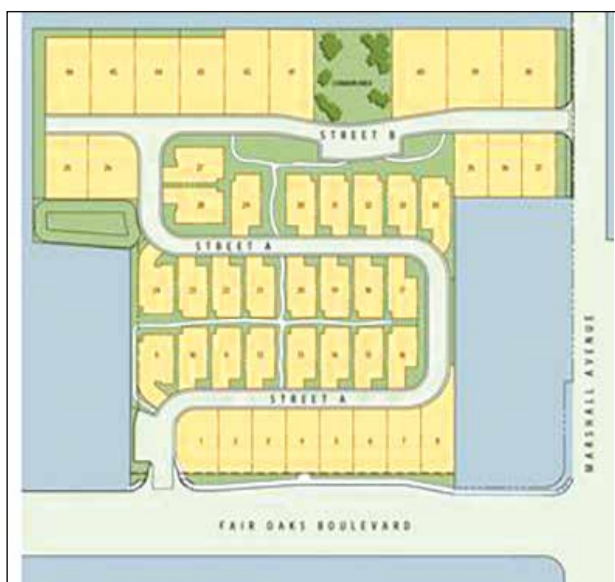
A diagram of The Paseos development includes larger perimeter lots and inner street sites for smaller “patio homes”. Courtesy of Homes By Towne.
