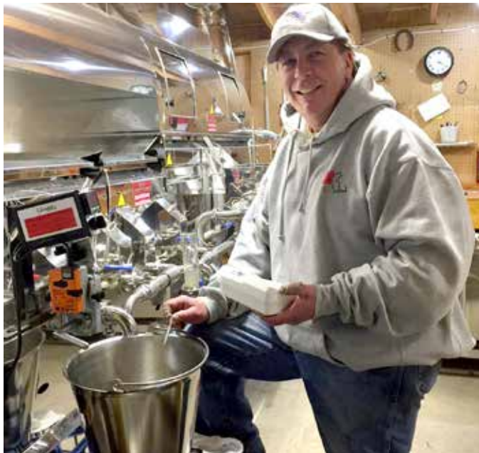
Quisset Hill Farm’s John Gomersall boils sap and measures its sugar content, which must be between 67 percent and 68 percent to avoid spoilage or crystallization. Courtesy photo
