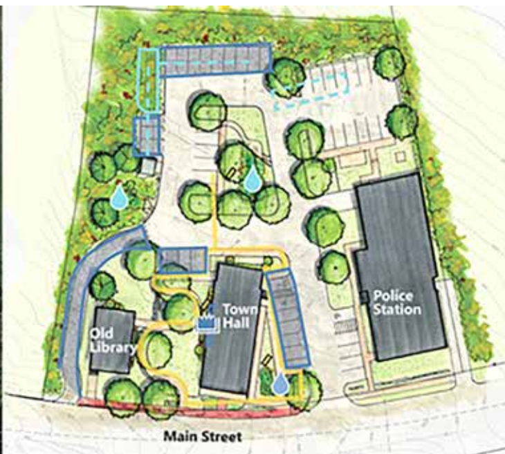
Mendon Town Hall campus before the redesign and a rendering by the Horsley Witten Group showing the area after paved surfaces are replaced by permeable surfaces and plantings. Source: www.mendontownhallcampusgreenguide.com
