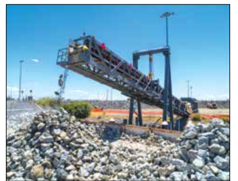
Rock is loaded onto barges at the California Department of Water Resources Weber Rock Yard near the Port of Stockton, California. The purpose of the rock barrier is to prevent the Delta from becoming too salty for irrigation, drinking water, or fish. Photo by Florence Low/California Department of Water Resources
