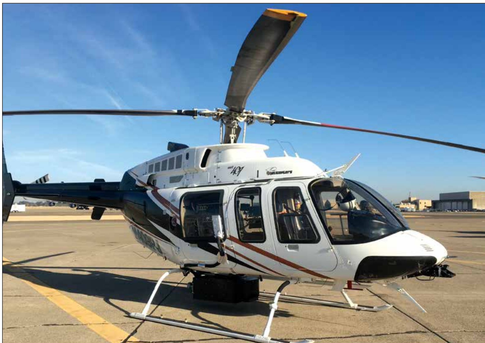
LIDAR technology and orthoimagery equipment mounted under the helicopter enables SMUD to identify potential fire threats and enhance its system reliability. Courtesy of SMUD
