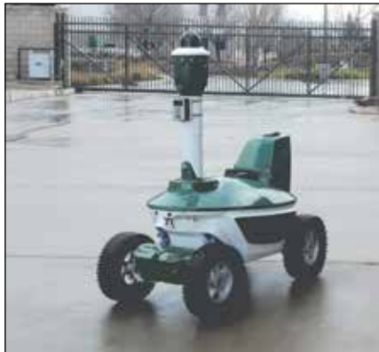
The RAD (Radio Activated Drone) monitors security and provides 24-seven surveillance patrol during emergencies and natural disasters, one of the "cool tools" offered by Verizon's Rocklin-based Emergency Response Team.
