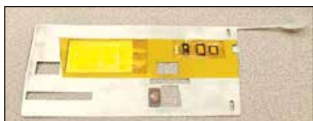
This card skimming device was removed from the Bank of America ATM in Gridley. Photo courtesy of Gridley Police Department
