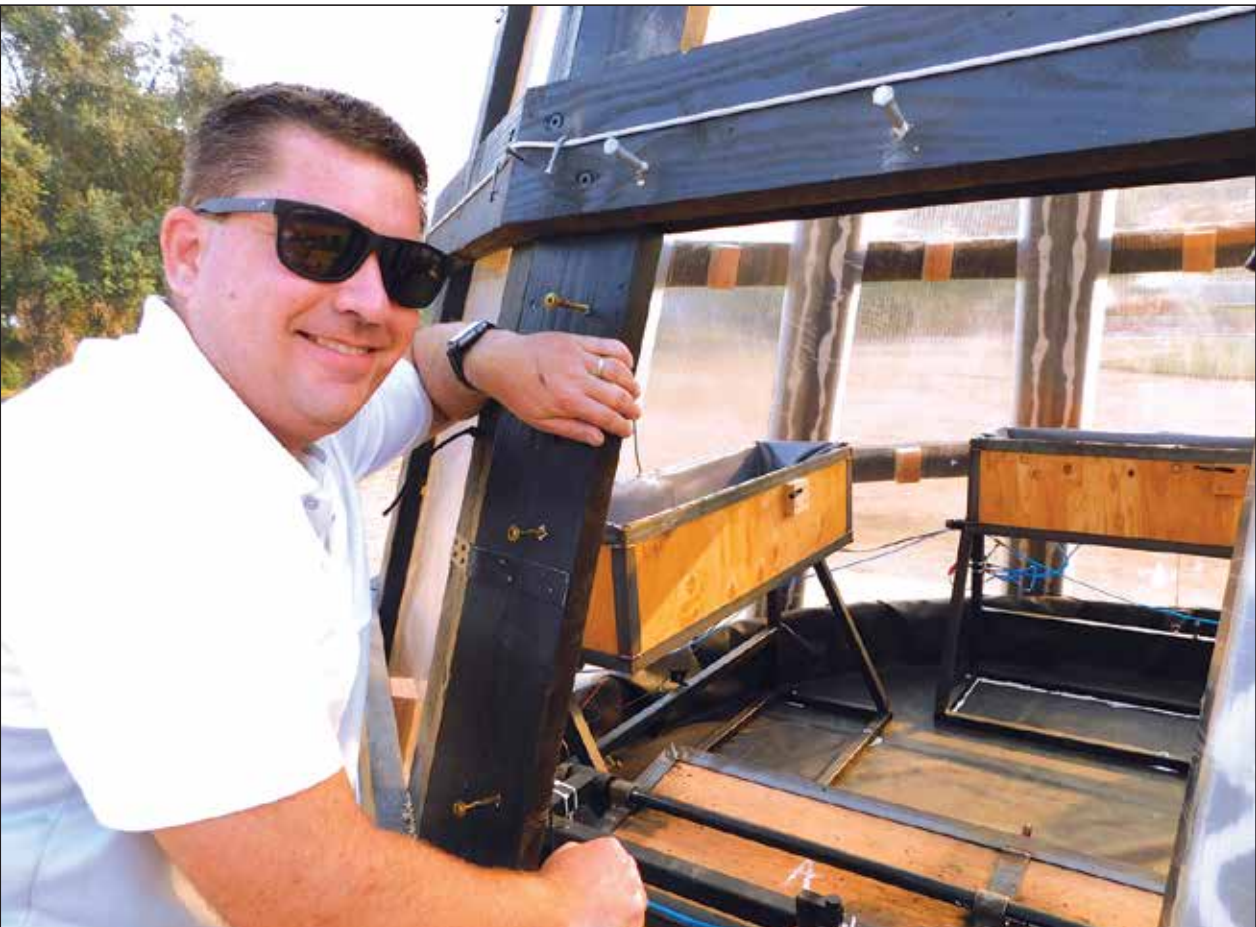
Belly of the Beast: Rober’s brother, Brian Rober, gives us a look inside the 20’ tall structure. At the push of a button, the square troughs seen will dump their load into the base of the structure, causing a chemical reaction so fast and hot that it could kill a man. The result was expected to blast steaming red foam 100’ into the air. Photo by Seti Long
