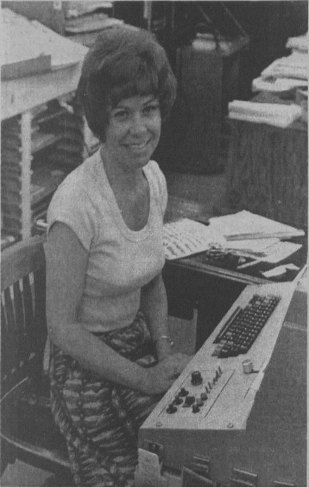
AN EARLY TYPESETTER FOR PHOTO OFFSET —Loretta Burks Carroll, the Herald's advertising director at the time, operates a first generation Compugraphic 7200 photo offset typesetting machine. It set single lines of type on strips of photographic paper for use as headlines and in ad composition.
