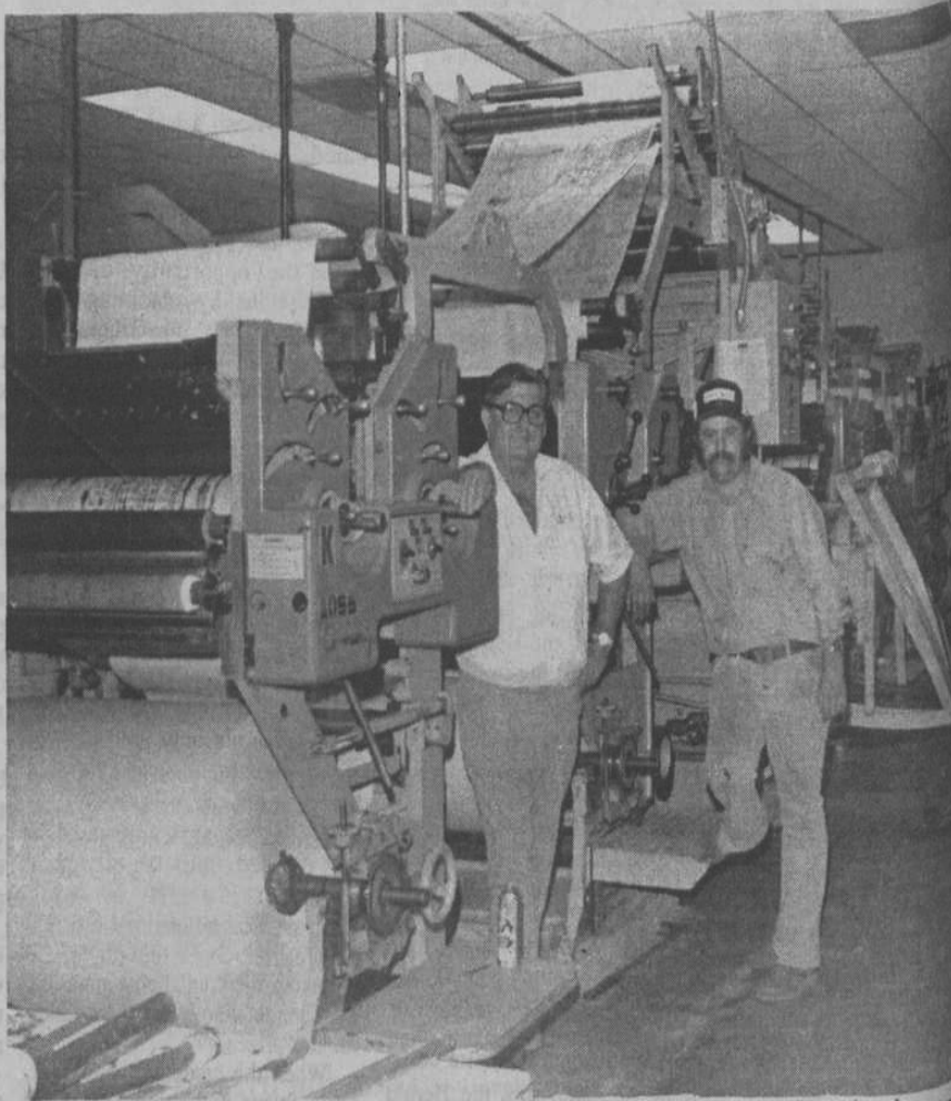
A HIGH-SPEED ROTARY PRESS —This is the Gridley Herald's Goss Community rotary press in August, 1980 when it had only six four-page units. Since then a seventh unit has been added and the Herald can now print a 28-page edition at one time. Today the press can run at 16,000 impressions an hour. With William David Burleson, left, in this photo is John Staley, Herald's production manager. When Burleson converted to the offset printing process in 1980, the press started with only two four-page units and a folder.
