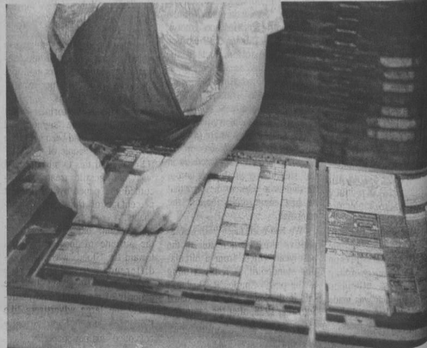
PLACING THE TYPE IN THE CHASE —After the lines of type cast by the Linotype were proofread and corrected, they were arranged where needed in a metal chase and inserted between the columns. After all the lines of type were in place, leads and slugs less than type high, were inserted to fill out the columns. Then it was all tightly locked using metal or wood spacers called furniture and special ratchet-like devices called quoins which had been seen in the foreground of this photo. The completed page of type was referred to as a galley when it was ready to be placed on the bed of the press.
