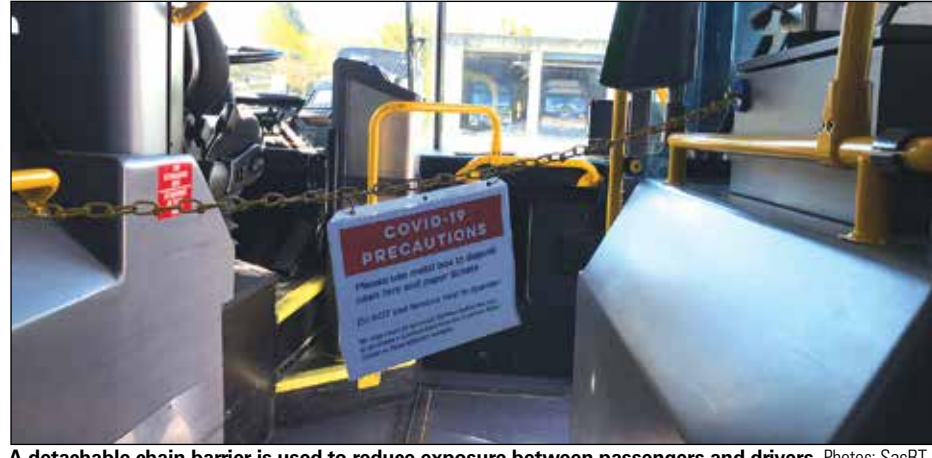
A detachable chain barrier is used to reduce exposure between passengers and drivers. Photos: SacRT
