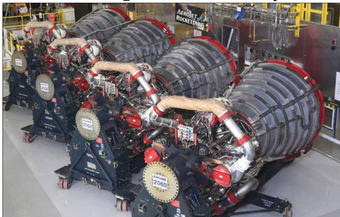
Aerojet Rocketdyne displays the four RS-25 engines slated to fly on EM-1, the maiden flight of NASA's SLS rocket, at its facility located at NASA's Stennis Space Center. Photo courtesy Aerojet
