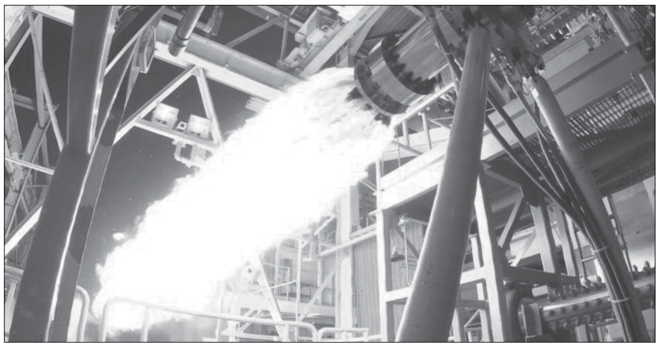
Staged-combustion testing at NASA's Stennis Space Center in Mississippi for the AR1 program is being developed by Aerojet Rocketdyne. Photo courtesy Aerojet Rocketdyne
