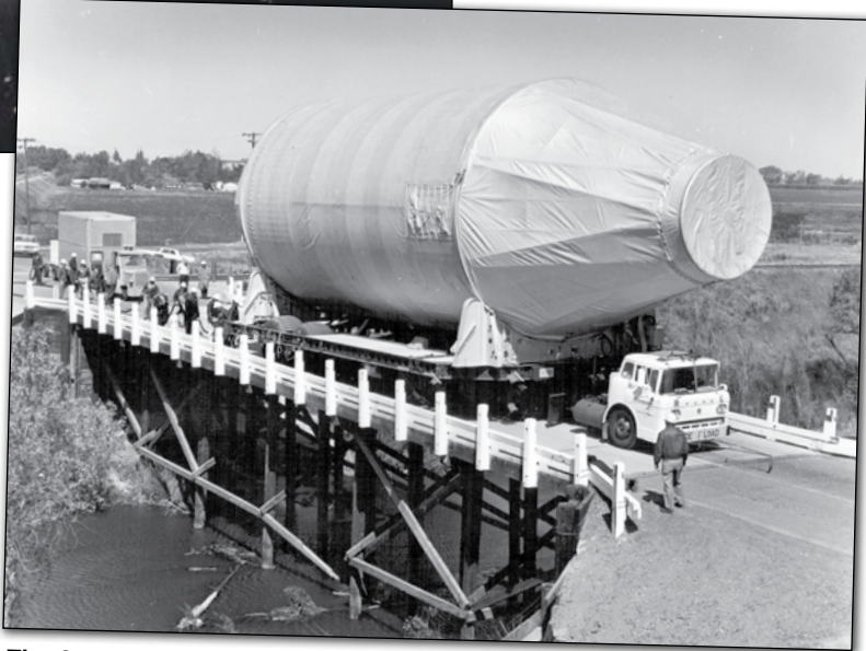
The S-IVB stages travelled from the Bay Area up the Sacramento River on barges. Once they arrived at the specially built dock in Hood, they were transferred to flatbed trailers for the trip to the test site traveling at seven miles per hour on narrow county roadways and bridges. Workmen along the route had to lift telephone wires and trim trees to enable the stage to make the journey to the test center. Photo courtesy of Center for Sacramento History, Douglas Aircraft Company/NASA Employee Collection, 2014/015.
