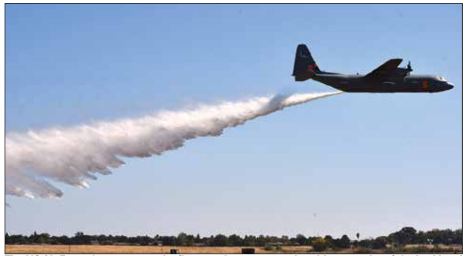
The US Air Force demonstrates the fire-containment, water-bombing capacity of the Lockheed C-130 Hercules. Photo by Rick Sloan
