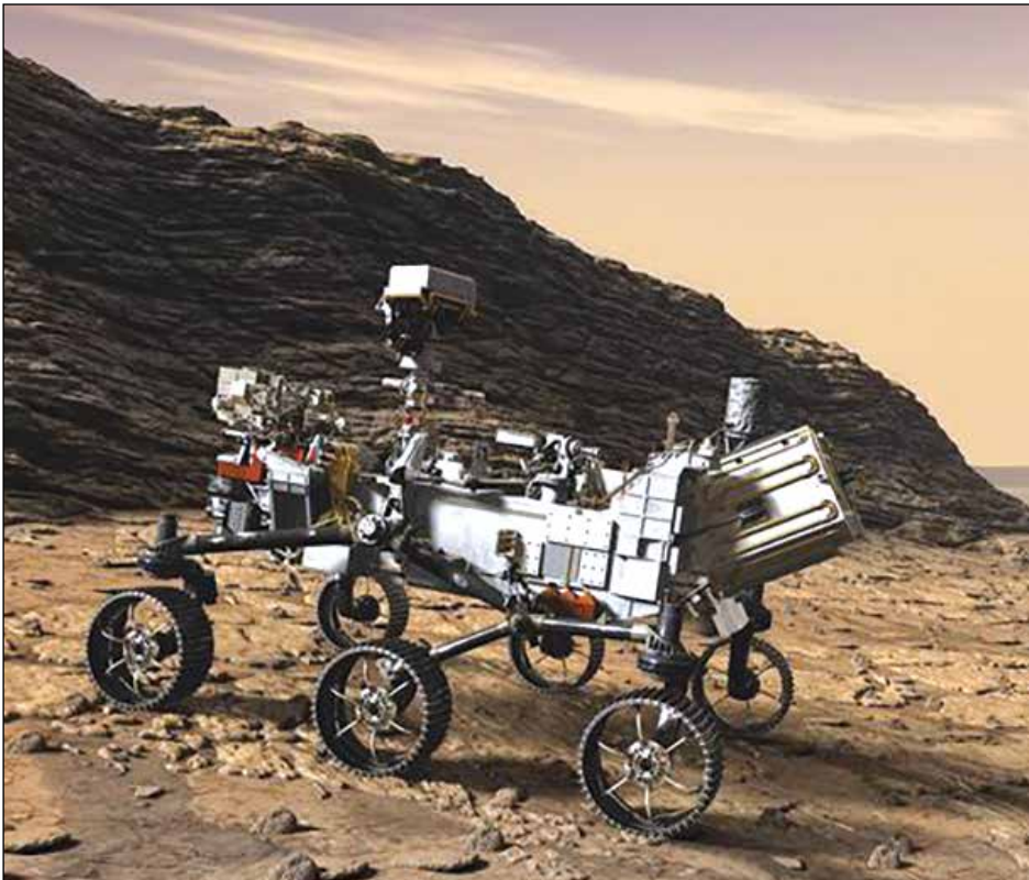
Artist's concept of NASA's Perseverance Rover. Perseverance's power source, a Multi-Mission Radioisotope Thermoelectric Generator (MMRTG) provided by Aerojet Rocketdyne, is visible at the aft end of the rover. Image Credit: NASA/JPL-Caltech
