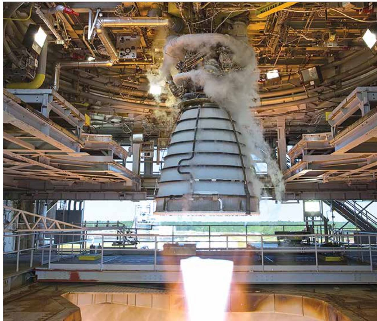
Aerojet Rocketdyne's RS-25 engine roars to life on the A-1 Test Stand at NASA's Stennis Space Center in Mississippi to test a new controller. Four RS-25 engines power the core stage of NASA's Space Launch System, the world's most powerful rocket. Photo taken Aug. 13, 2015. Photo: Aerojet Rocketdyne
