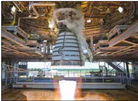
Aerojet Rocketdyne’s RS-25 engine roars to life on the A-1 Test Stand at NASA’s Stennis Space Center in Mississippi to test a new controller. Four RS-25 engines power the core stage of NASA’s Space Launch System, the world’s most powerful rocket. Photo taken Aug. 13, 2015. Photo: Aerojet Rocketdyne
