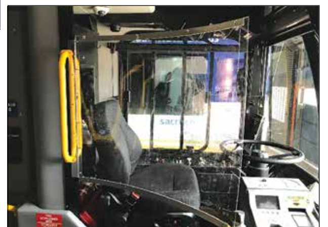
Above: A detachable chain barrier is used to reduce exposure between passengers and drivers. Right: SacRT is currently installing a protective plexi-glass barrier on each bus by the driver's seat. Photos: SacRT
