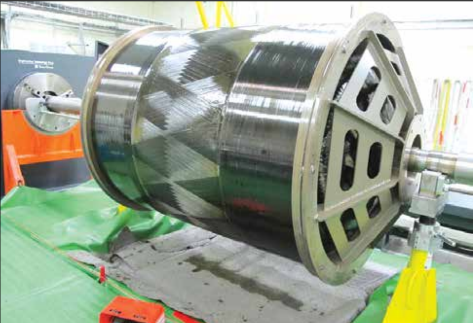
An example of the type of large solid motor carbon fiber case Aerojet Rocketdyne will produce at its new Huntsville, Alabama, Advanced Manufacturing Facility starting in early 2020. Aerojet Rocketdyne photo
