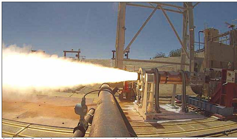
An Aerojet Rocketdyne solid rocket motor that had been conditioned to mimic an extreme cold-soak condition for air-launch application recently completed successful hot-fire testing at AFRL at Edwards Air Force Base in California
