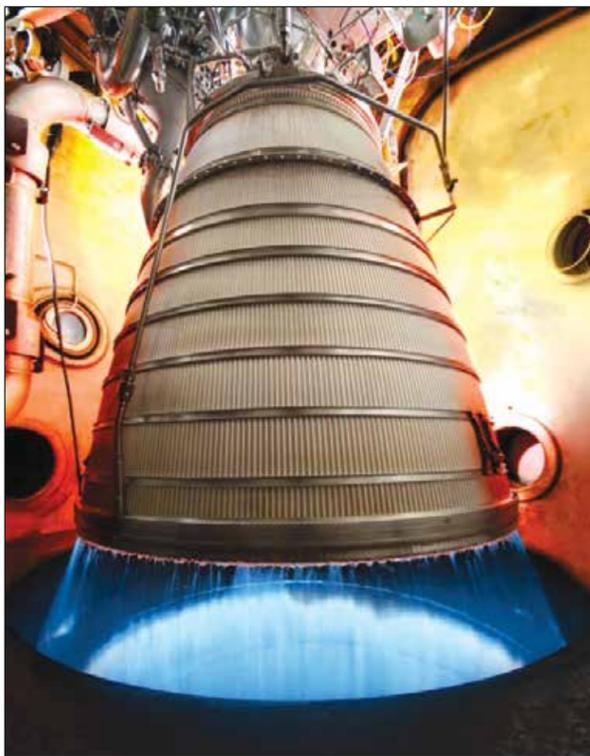
NASA's InSight Mars lander mission will be using the United Launch Alliance Atlas V, whose Centaur upper stage is powered by a single Aerojet Rocketdyne RL10C-1 engine (shown here). It is powerful enough to launch planetary probes from either U.S. coast, depending on their mission mass. Photo courtesy Aerojet Rocketdyne
