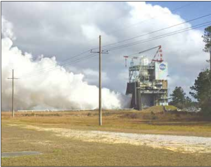
NASA and Aerojet Rocketdyne Test the RS-25 Engine for NASA's Space Launch System at Stennis Space Center. Photo courtesy of Aerojet
