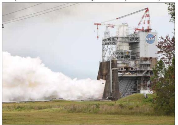
Aerojet Rocketdyne tests the third RS-25 flight controller on a developmental engine at NASA's Stennis Space Center on July 25, 2017. Photo courtesy Aerojet
