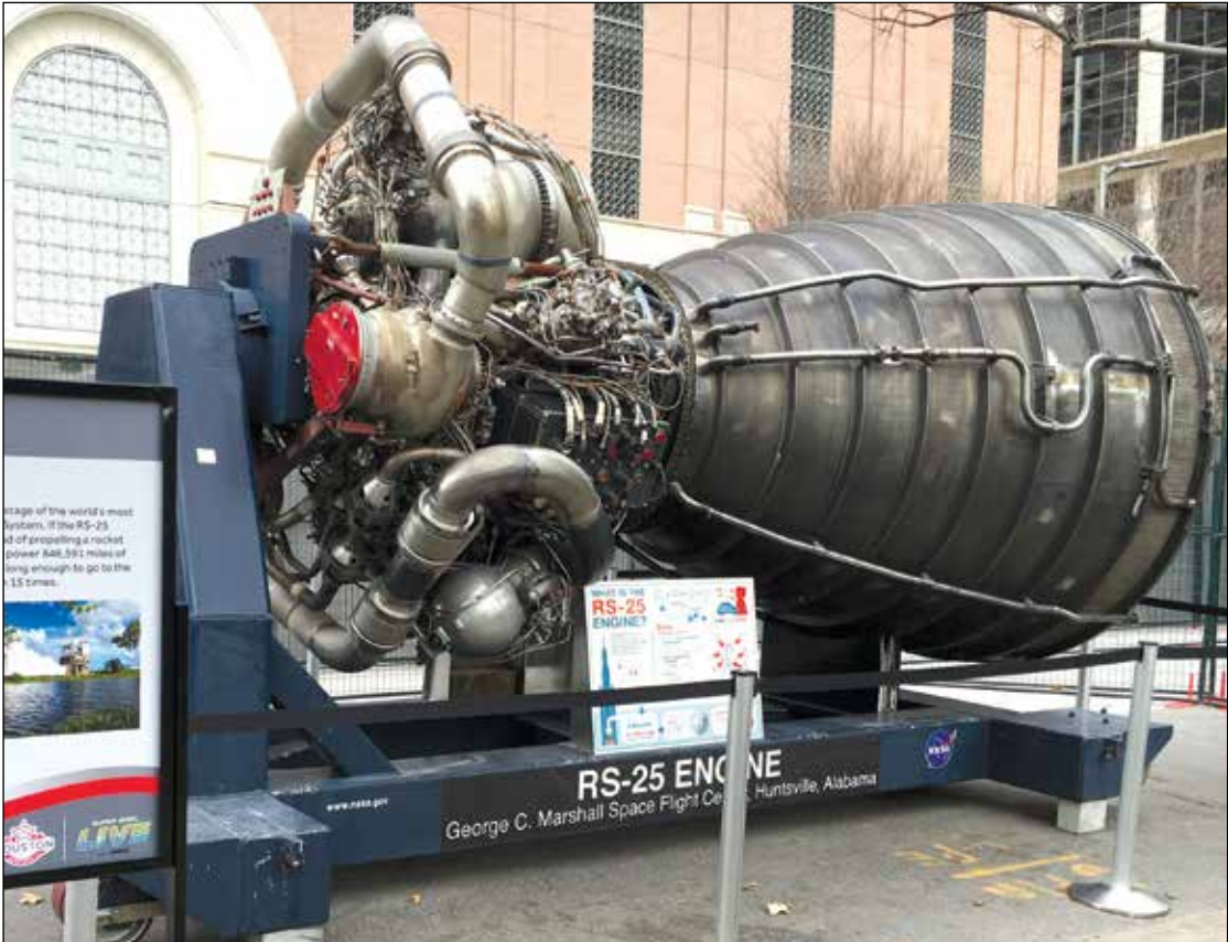
The RS-25 engine, developed and manufactured by Aerojet Rocketdyne, is on display at Future Flight in Houston, TX. Four RS-25 engines will power the core stage of the world’s most powerful rocket, NASA’s Space Launch System. Photo courtesy Aerojet Rocketdyne
