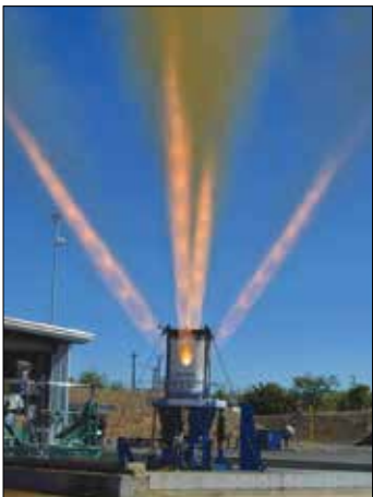
Third development jettison motor for NASA's Orion Launch Abort System fires for 1.5 seconds at Aerojet Rocketdyne's facility in Rancho Cordova, California.
