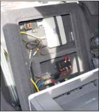
The custom networking system, hidden in what used to be the back passenger seat, enables Code Officers to connect directly to the City Hall network. They can access and share documents, go online, and receive faxes.
