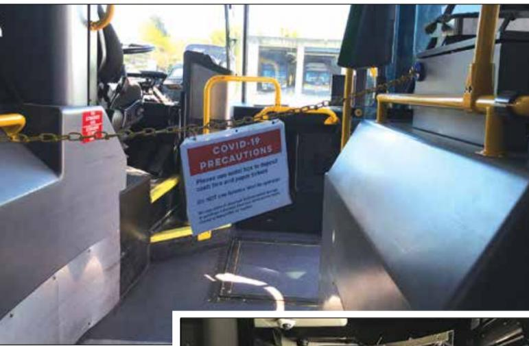
Above: A detachable chain barrier is used to reduce exposure between passengers and drivers. Right: SacRT is currently installing a protective plexi-glass barrier on each bus by the driver's seat. Photos: SacRT
