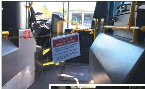
Above: A detachable chain barrier is used to reduce exposure between passengers and drivers. Right: SacRT is currently installing a protective plexi-glass barrier on each bus by the driver's seat. Photos: SacRT
