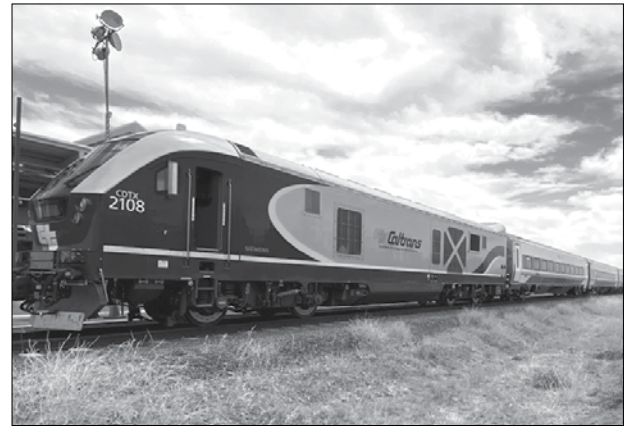
Charger locomotive leading a Siemens Mobility Venture trainset. Photo courtesy of Caltrans
