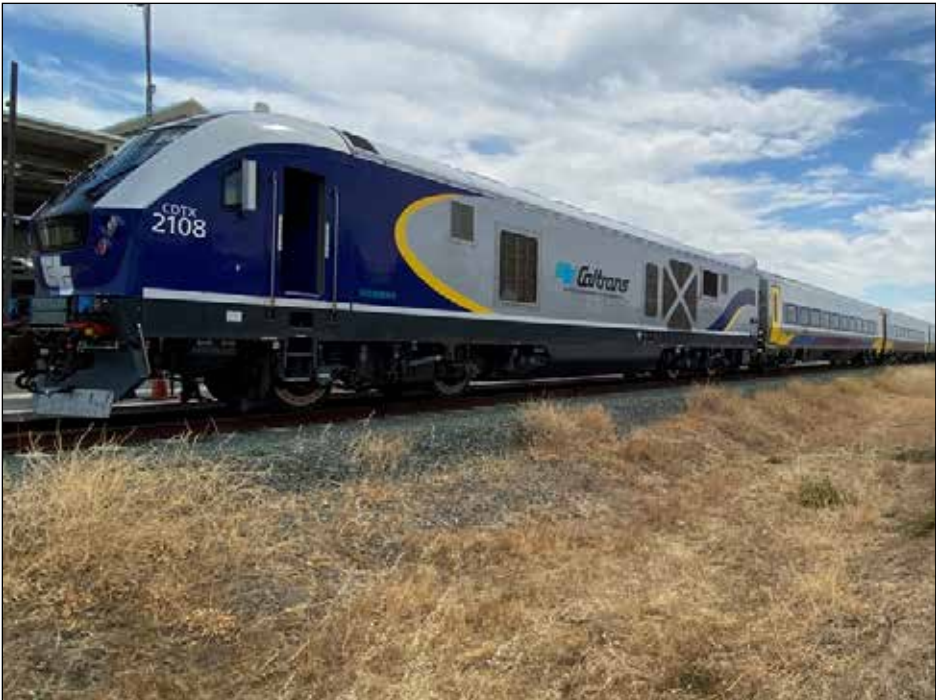
Charger locomotive leading a Siemens Mobility Venture trainset. Photo courtesy of Caltrans
