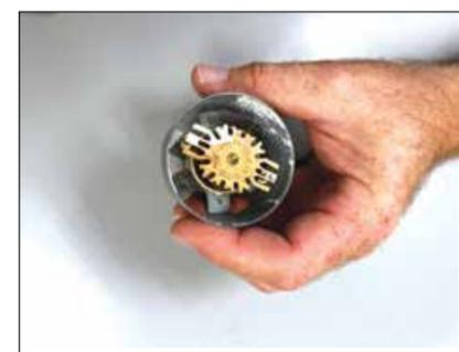
Malone held a sprinkler head with a dab of paint on it that would prevent it from getting proper signal and reaction if there was a fire.
