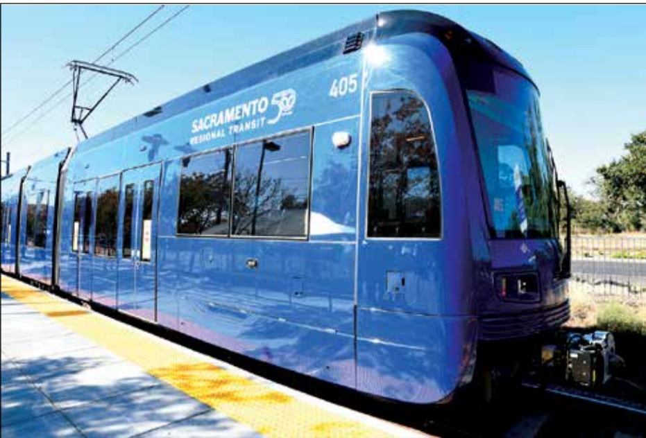
SacRT is testing 17 new low-floor trains built at Siemens Mobility in south Sacramento, modifying station platforms along the Gold Line to meet the height requirements. Photo courtesy of SacRT
