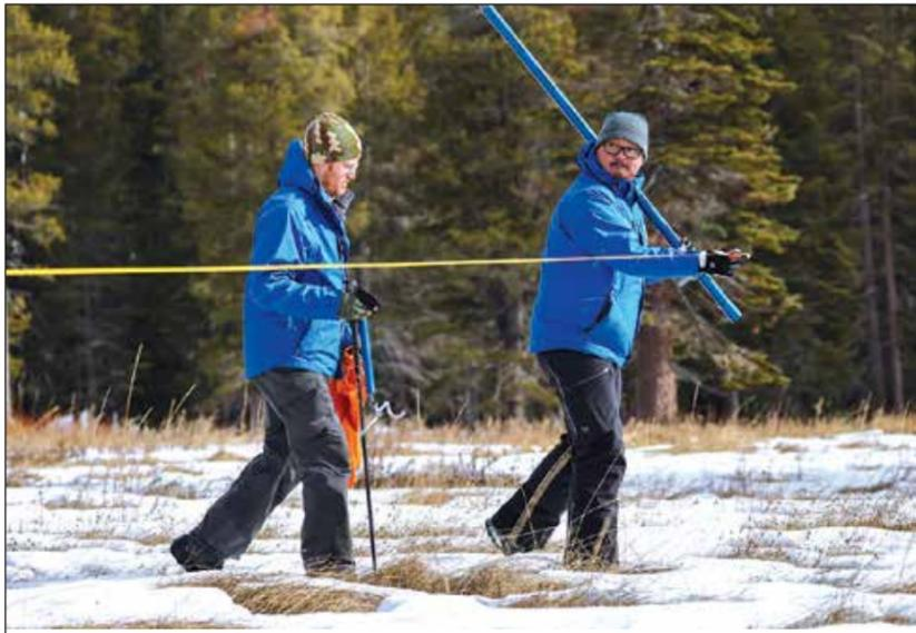
The Department of Water Resources (DWR) conducted the first snow survey of the season on January 2, 2023, at Phillips Station. The manual survey recorded 7.5 inches of snow depth and a snow water equivalent of 3 inches, which is 30 percent of average for this location. Photo courtesy of DWR
