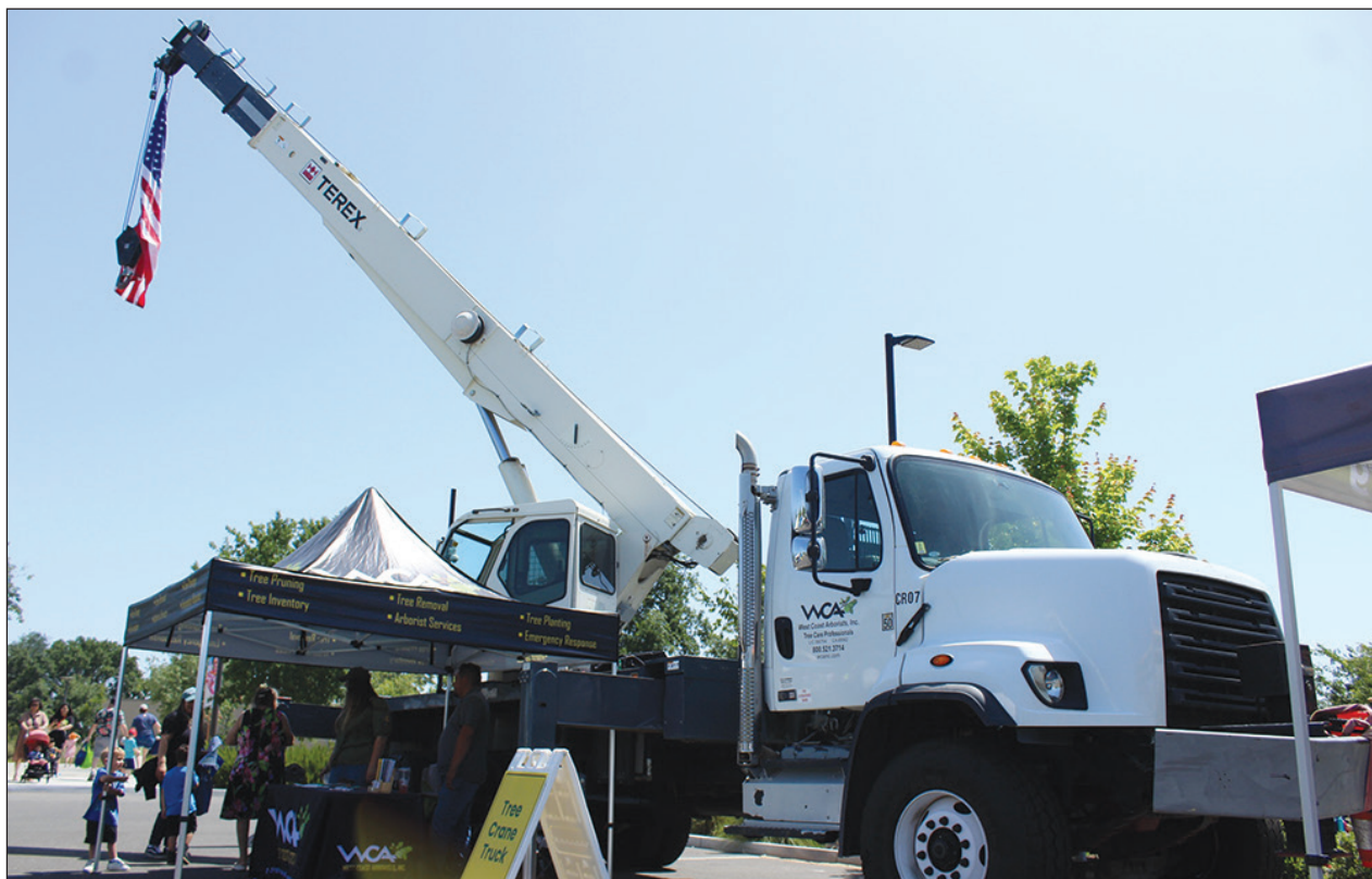
West Coast Arborists uses its crane truck to remove trees that would be unsafe to cut down. The vehicle can lift up to 28 tons. Photos by Matthew Malone
