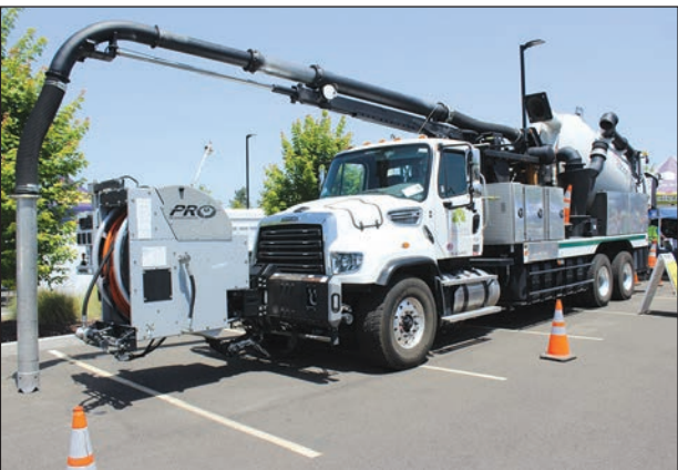
The city of Elk Grove's vacuum truck is used to clean storm drains and prevent flooding in the rainy season.
