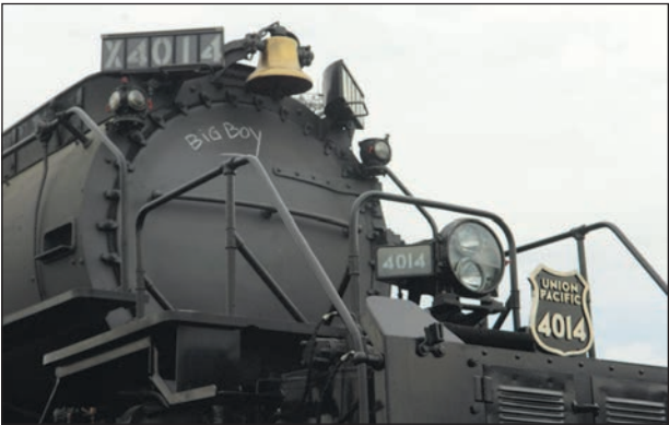
Union Pacific's 4014 Big Boy, an oil-burning 4-8-8-4 locomotive, is 132 feet long and weighs 1.2 million pounds.
