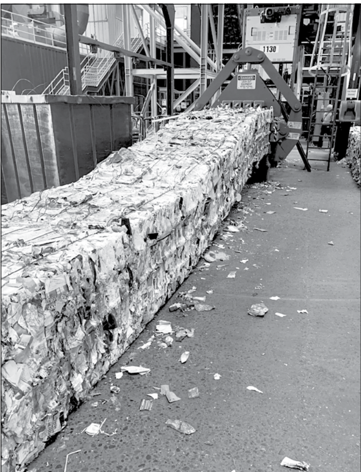
★ Pictured here is WM’s processing facility, compacted and baled mixed paper with cartons. Photo courtesy of Yolo County
