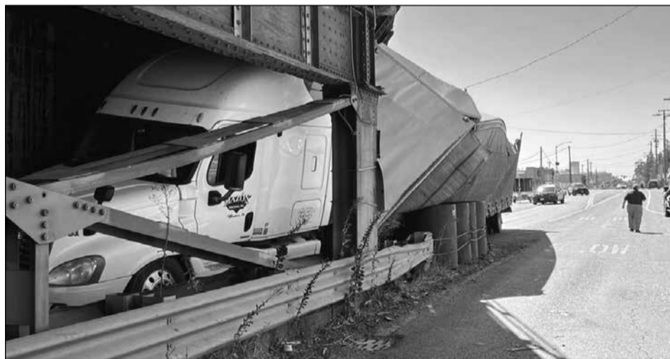
Planned improvements to State Route 70 include increased railroad bridge clearances. Photo courtesy of California Department of Transportation
