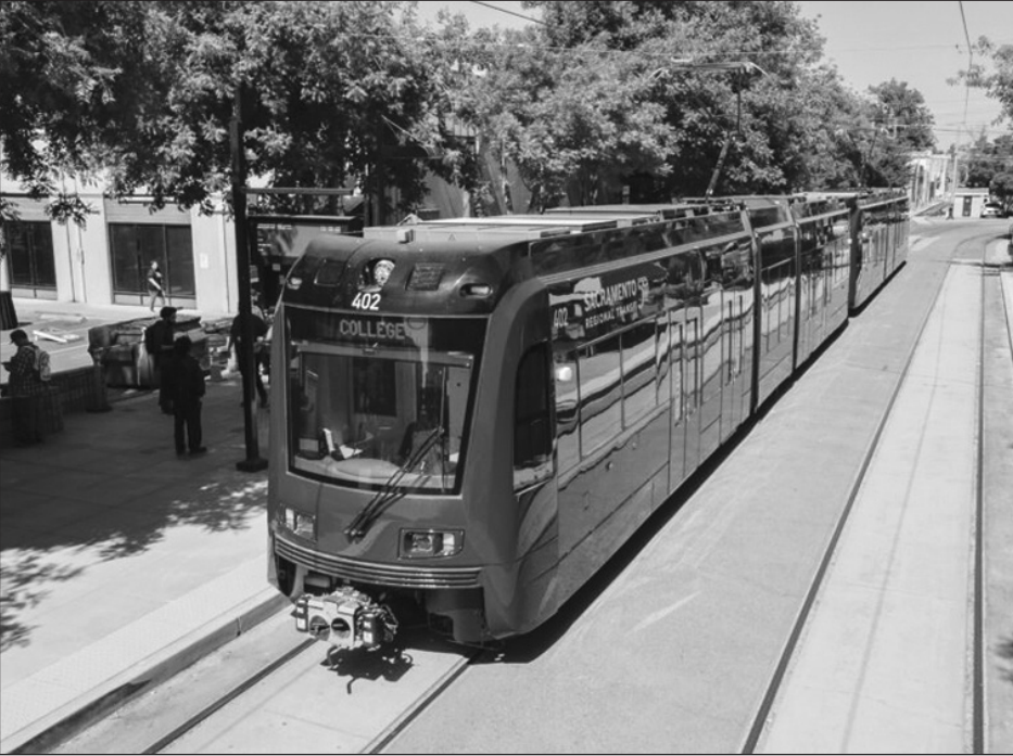
The S700 low-floor light rail trains are designed to enhance accessibility, comfort and efficiency for all riders. Photo courtesy of SacRT
