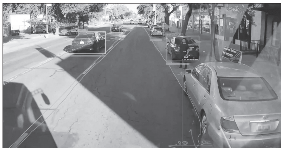
Pictured is the view from forward-facing cameras on SacRT buses that use artificial intelligence to detect parking violations within the City of Sacramento. Photo courtesy of SacRT
