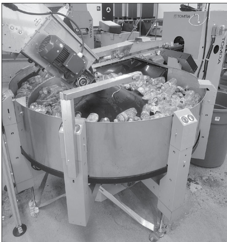
Simply Recycle is powered by TOMRA technology. Shown here is the automated sorting and weighing machine.
