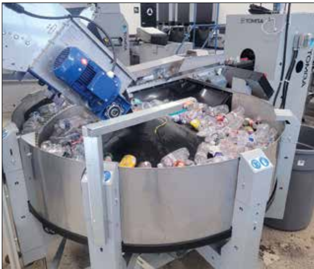
Simply Recycle is powered by TOMRA technology. Shown here is the automated sorting and weighing machine.
