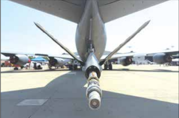
The boom of a KC-135 Stratotanker sits fully extended, an uncommon sight during static displays, allowing guests a close-up look at the in-flight refueling system usually only seen by fellow pilots midair. Photo by Shamaya Sutton
