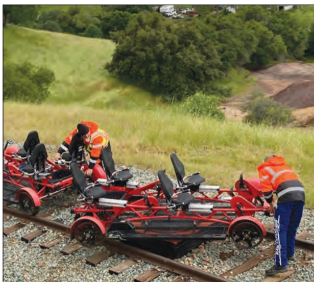
Rail Explorers staffers turn the railbikes on an air-powered lift before the downhill return trip.
